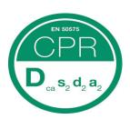
Instrumentation cable for fixed installations indoors and outdoors. Not to be laid in soil nor directly in cast concrete. Installations must be in accordance with national regulations and rules of installations. The cable is halogen-free and flame-retardant according to CPR-class Dca-s2,d2,a2.
