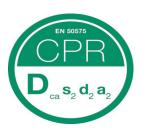
Installation wirefor fixed installations indoors. For internal wiring of electrical devices. The conductor insulation must be protected against UV-radiation. The cable is halogen-free and flame-retardant according to CPR-class Dca-s2,d2,a2.
